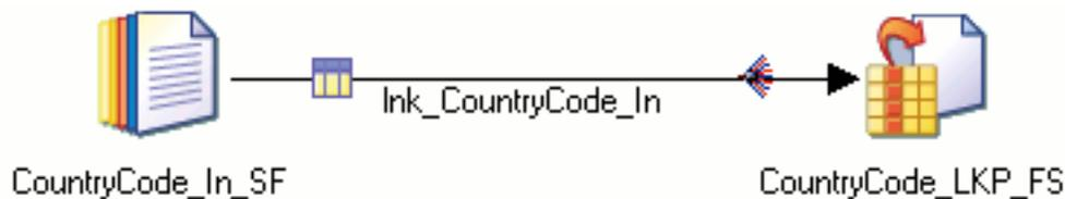
Figure 2. Your first job is composed of a Sequential File stage that writes to a Lookup File Set stage.
